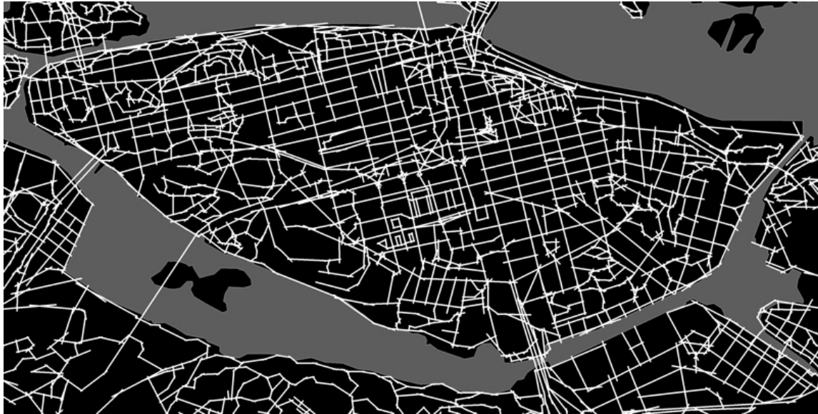
Fig. 3. The axial map: a network representation of urban spatial form, constructed by the least amount of straight lines that cover all public open space, where the axial line represents a space that is possible to visually overlook and physically access for an experiencing person in the street.
